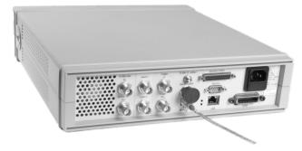
The USB interface requires no front panel configuration. USB operation and configuration is supported by the version of *VISA and SICL I/O libraries* on your computer.
