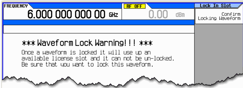
Figure 8-37 Waveform Lock Warning
