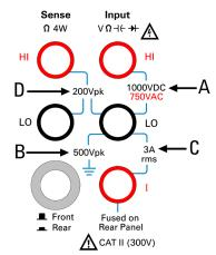
**Note:** The front-panel terminals are shown above. The rear-panel terminals are identical. The Front/Rear switch selects the terminal set to be used. *Do not operate this switch while signals are present on the front or rear terminals*. The current-protection fuse is on the rear panel.
