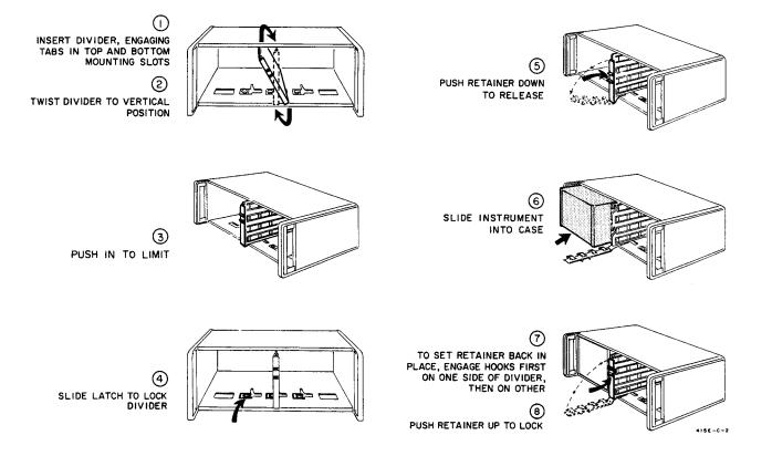
Figure 2-2. HP Model 1051A Combining Case Instrument Installation
