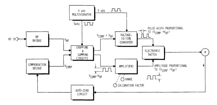
Figure 4-1. Simplified 432A Block Diagram
