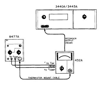
Figure 5-1. Check and Adjustment Test Set-Up
