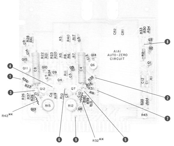
Figure 7-7. A1 Bridge Assembly Component Locations
