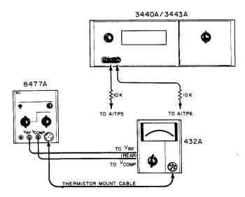
Figure 5-3. Bridge Amplifier Test
