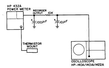
Figure 5-2. Zero Carryover Test Setup
