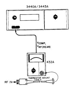
Figure 3-1. Precision Power Measurements
