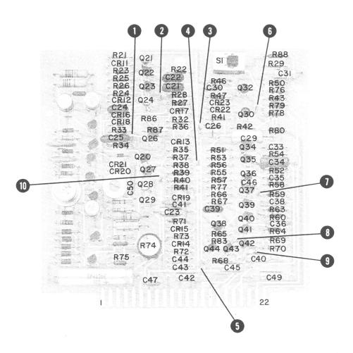
Figure 7-11. A2 Meter Logic Assembly Component Locations
