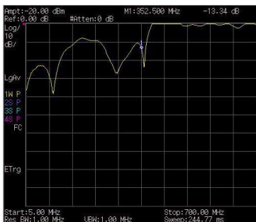
Figure 4-22 Measuring the Return Loss of the Filter
