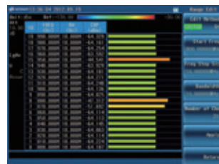
N9322C - Channel Scanner (信道扫描) 可同时扫描 20 个信道, 并测量信道功率
