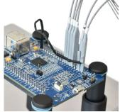
For headers with signals situated together and not enough grounds. A ground lead can be used to connect to a remote ground pin on the device under test.
