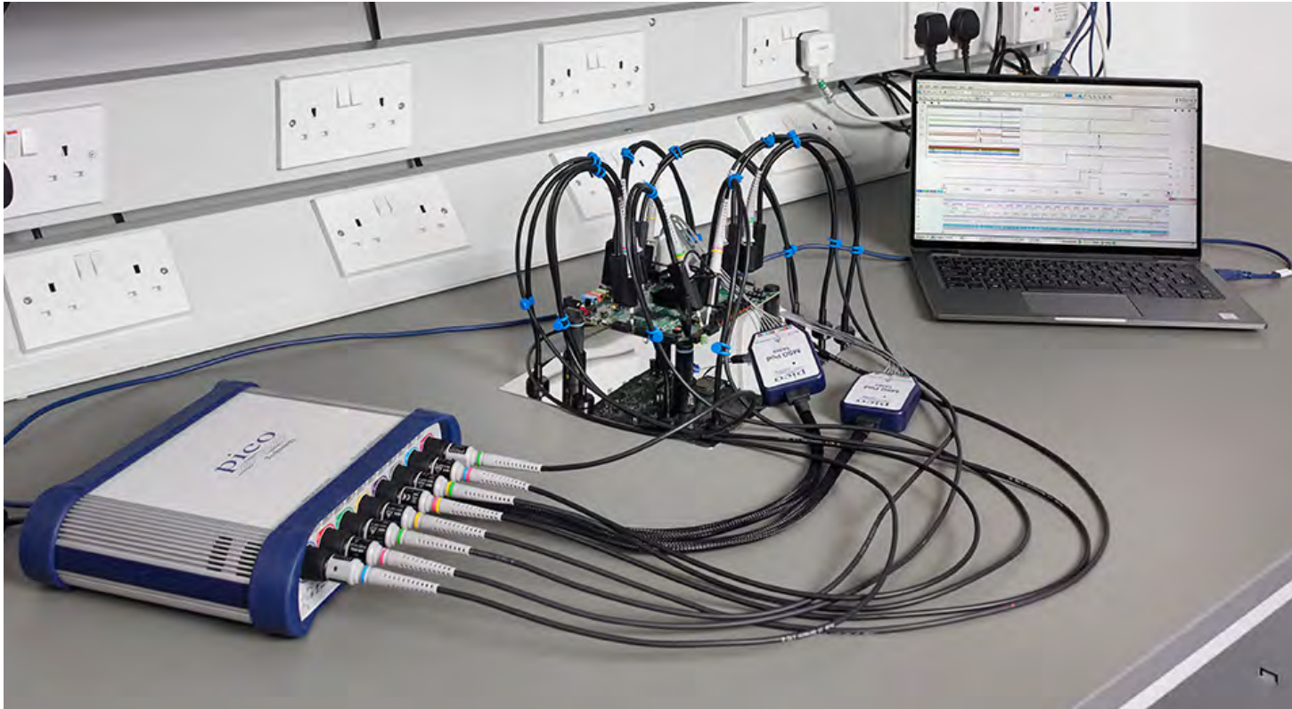
The PicoScope 6000E Series oscilloscope utilizing all eight analog channels and all 16 MSO channels. All the analog probes are situated on the device under test (DUT) and held in place by the probe positioning kit (available separately).
