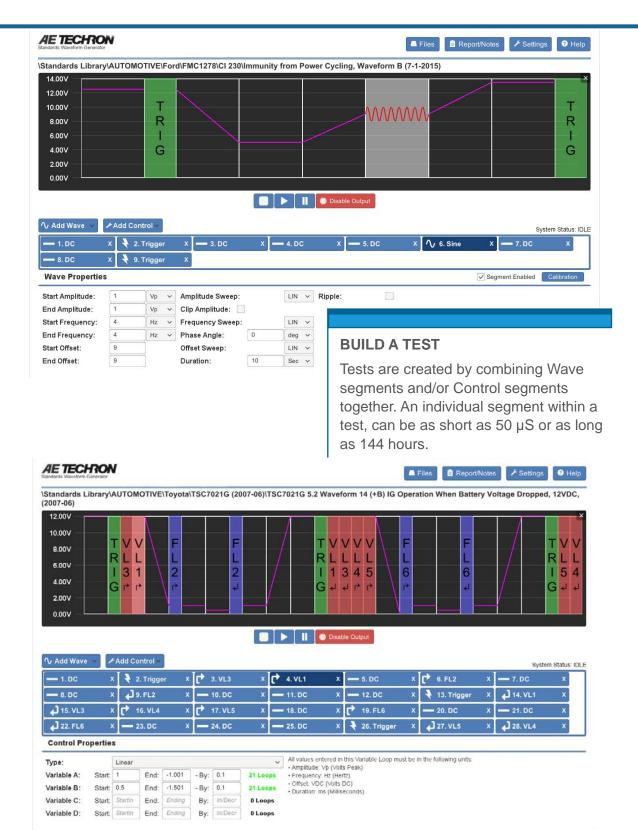
**WAVE CONTROLS** like Fixed Loop, Variable Loop, and Trigger make the 3110A able to reproduce very complex standards.
