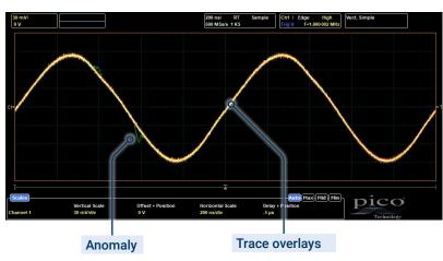
Having captured an anomalous event you can scroll through, or close gates around, an ever smaller block of overlaid traces, until the anomalous trace or traces are found. There is also a segment finder which uses a binary search method to address larger numbers of trace segments:
