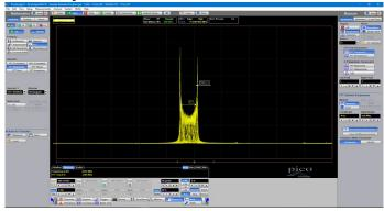
All PicoScope 9400 Series oscilloscopes can calculate real, imaginary and complex Fast Fourier and Inverse Fast Fourier Transforms of input signals using a range of windowing functions. The results can be further processed using the math functions. FFTs are useful for finding crosstalk and distortion problems, adjusting filter circuits, testing system impulse responses and identifying and locating noise and interference sources.
